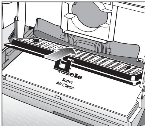
The "ACTIVE air clean" filter can be used instead of the "ACTIVE HEPA" filter and vice versa. Remember to reset the filter change indicator with the Reset button after every filter change.
